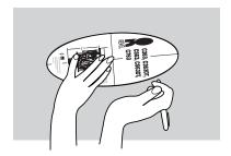
Cut the ceiling drywall along the mark you made in Step 2 to create the mounting opening.
