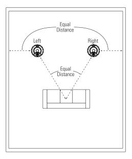
Ideally, the distance between the left and right loudspeakers should be slightly less than their distance from the primary listening area.
